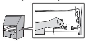
Being careful not to contact the CRT assembly, slide the top portion of the cabinet back slightly.
